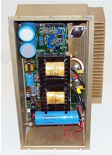
Fig. 1. Photograph of d.c. power heater supply of CX unit
