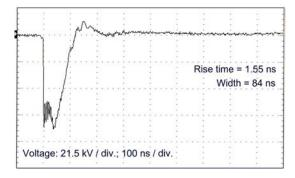
**Figure 3.** Voltage waveform obtained with the Marx Generator and 50  $\Omega$  resistor. Here, a simple peaking circuit is present. For other application, the peaking circuit currently employed can be kept and a vacuum diode assembly introduced to yield pulsed X-ray system suitable for flush X-ray photography.
