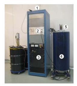
**Figure 1**. Experimental set-up. (1) Hand held 80 V trigger, (2) 50 kV trigger circuit, (3) Controller of 40 kV-40 mA DC Power Supply, (4) 30-stage inductively charged Marx Generator with the peaking capacitor, and peaking spark gap and (5) Load. This load can be either the MCG-like coil, the oscillatory circuit with the gas discharge switch assembly, BWO or the X-ray diode. DC Power Supply barrel and the charging barrel are placed on the left of the cabinet.
