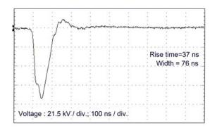
**Figure 2**. Voltage waveform obtained with the Marx Generator and 50  $\Omega$  resistor. The peaking circuit is absent.
