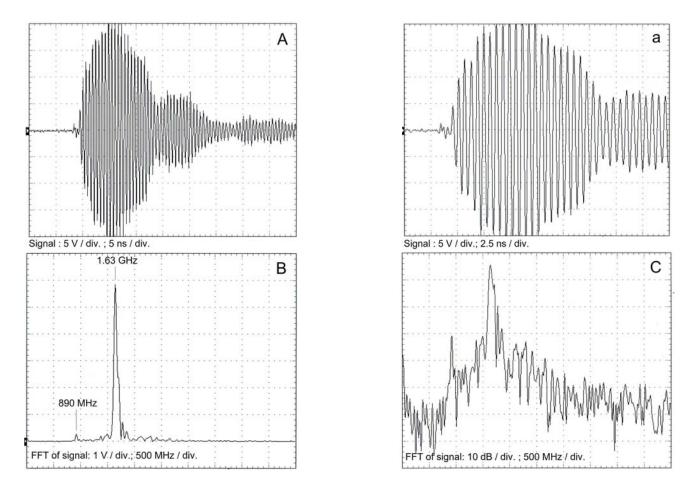
**Figure 4**; Experimental data; **Frame A**: Signal recorded at the time scale of 5 ns per division. **Frames B** and **C** are the FFT of the signal, shown on the linear and logarithmic scale. **Frame a**: is the signal of the frame A, but expanded on the time scale of 2.5 ns per division. B-dot probe is used. For frequency of 1.63 GHz, the amplitude of the signal of 1 Volt measured by the probe corresponds to the electric field of 1.9 kV/cm.
