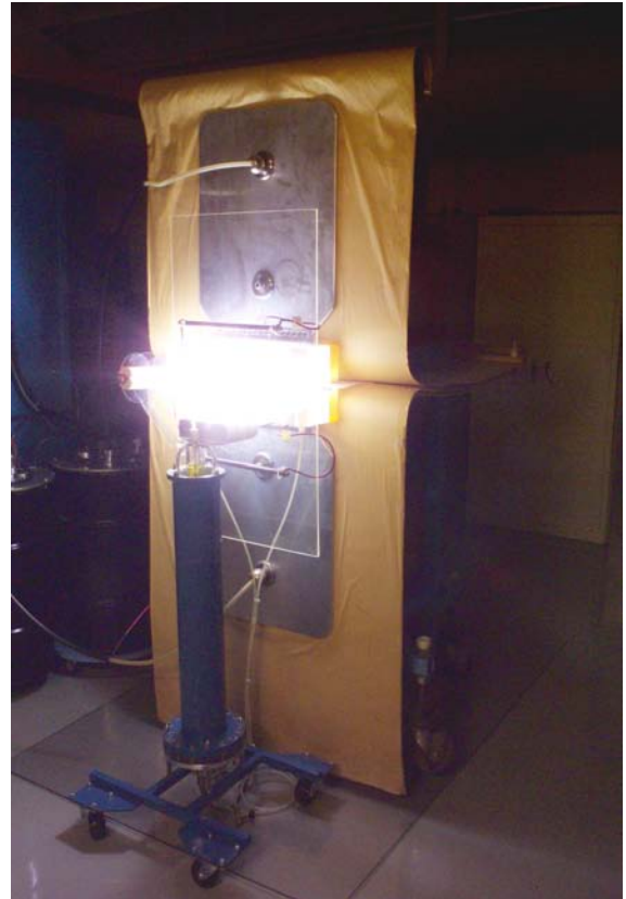
Figure 3. Photograph of 1/4 module in action. 250 kV pulse from the Mini-Marx generator triggers the 1/4 module
