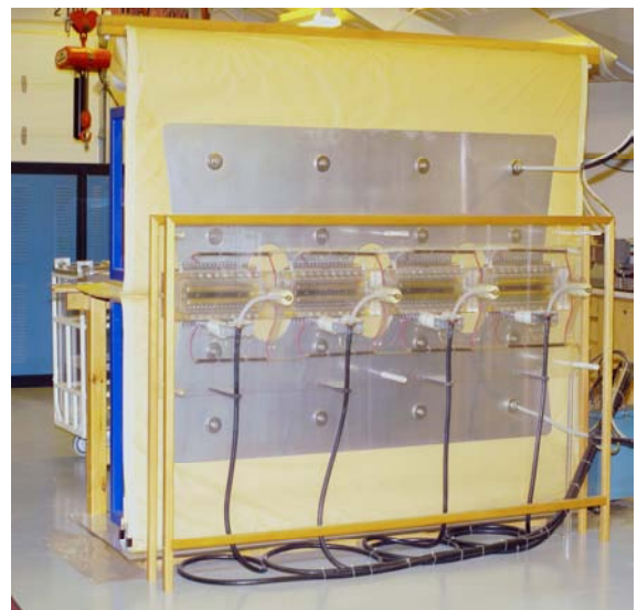
Figure 4. Photograph of module obtained by connecting four 1/4 modules in parallel
