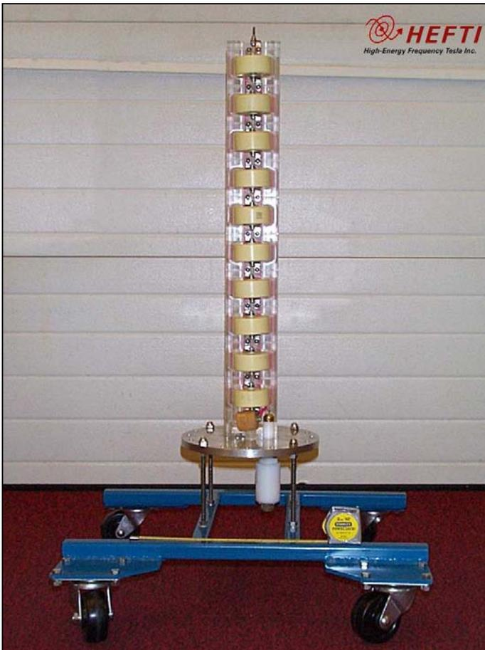
**Figure 1** Interior of 10-stage Mini Marx Generator
