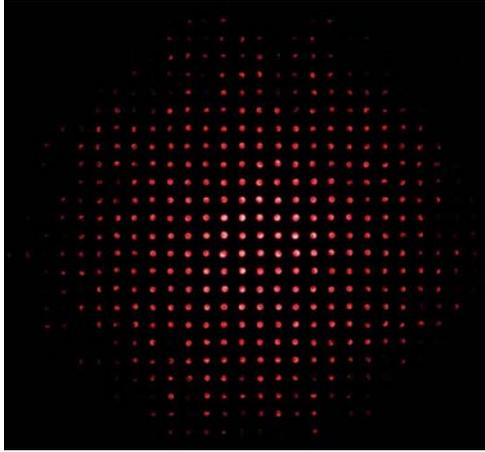
**Figure 4.** Ignition of the neon bulbs by the RF/HPM radiation
