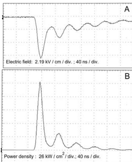
**Figure 6.** Frame A is the electric field, E recorded by E-field probe and frame B is the power density,  $E^2 / (120\pi)$ . Distance from the antenna to the probe, d is 40 cm.
