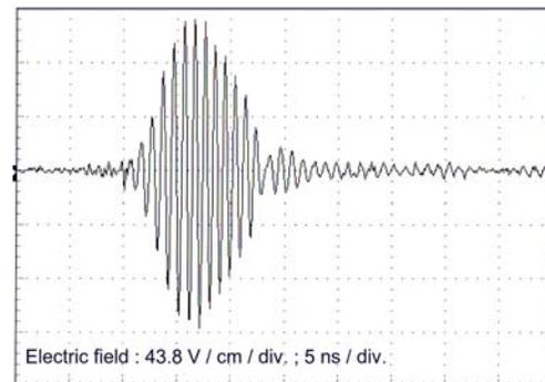
**Figure 8.** Electric field, E recorded with the electric field probe and 1 GHz high-pass filter at  $d=35$  cm. The product: E times d is constant from 35 cm to 2.5 m.
