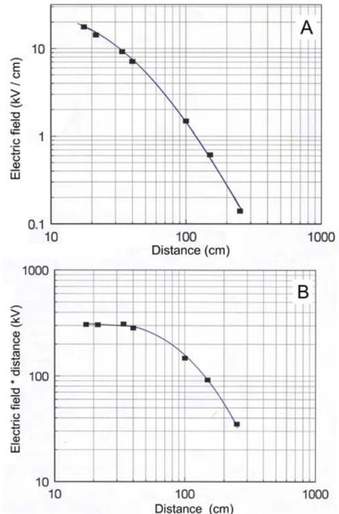
**Figure 7;** Frame A is the plot of the electric field, E in kV/ cm vs distance in cm. Frame B is the graph of the product of the electric field and distance vs distance. Here, E is recorded by E field probe.
