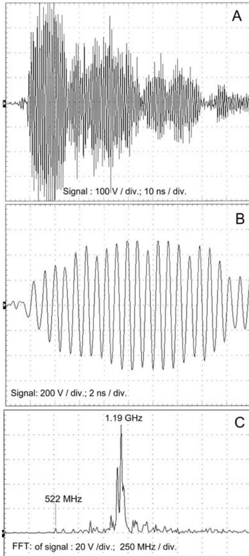
**Figure 2.** HPM pulse is recorded with the single turn loop probe of 1.89 cm in diameter. The probe is placed in the waveguide. The oscillatory circuit is tuned to produce the standing wave at 1.19 GHz. Frame B is the expanded waveform of frame A. FFT of signal is shown in frame C. Charging voltage is 33 kV/stage.
