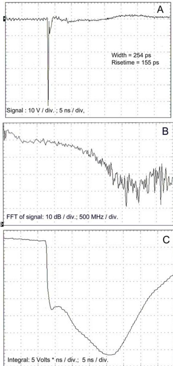
**Figure 5;** Data at 17 cm. Frame A is the B-dot signal. Frame B is the FFT of A. Frame C is the integral of the B-dot signal to get the magnetic field. B-dot probe is calibrated in the TEM-cell to obtain the electric field (=the integral of B-dot)
