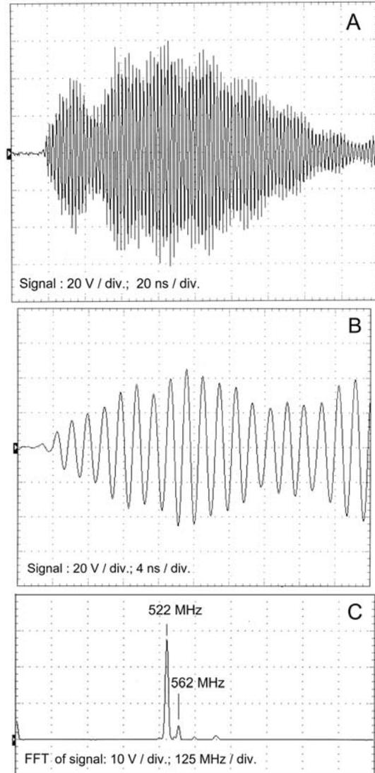
**Figure 3.** Experimental conditions are as in Figure 2, except that the oscillatory circuit is tuned to produce the frequency of 522 MHz. The waveguide is used as in Fig. 2. The data in Figure 3 are recorded with low-pass filter of 560 MHz.
