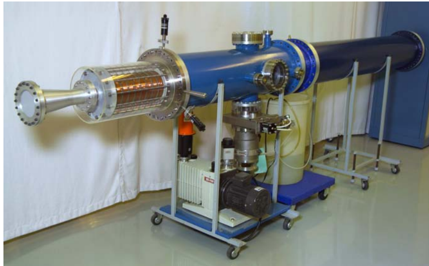
Figure 1. Photograph of 10 GHz BWO driven by 24-stage Marx generator
